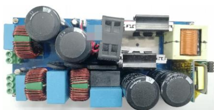
PFC Inverter Power Supply Solution
